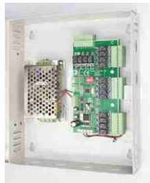
Multiple Elevator Control Box
