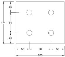
Glass Hole Diameter = Ø22mm
