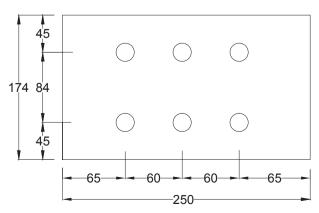
Glass Hole Diameter = Ø22mm
