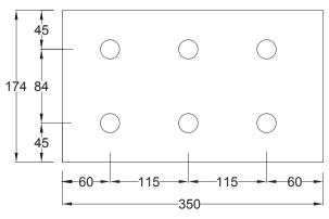
Glass Hole Diameter = Ø22mm
