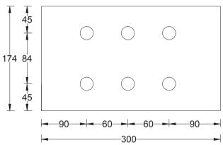
Glass Hole Diameter = Ø22mm
