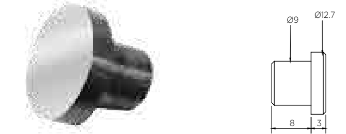
OZRAC - EC - 12A For Dia 12mmX1.5mm thick pipe SS-304 Grade SSS Finish Push Fit End Cap
