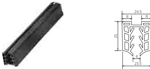
OZRAC - GKT - 22 24.5mmX 25mm (Flexible) EPDM Black Color For 10mm thick Glass
